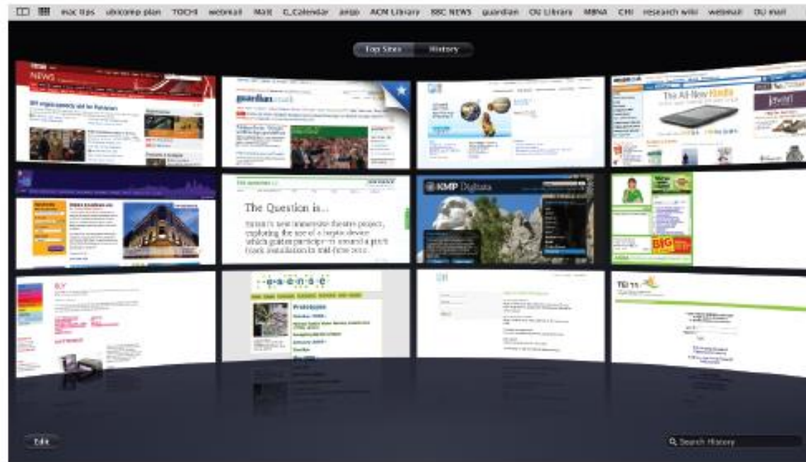
Figure 6.3 A window management technique provided in Safari: pressing the 4 \times 3 icon in the top left corner of the bookmarks bar displays the 12 top sites visited, by shrinking them and placing them side by side. This enables the user to see them all at a glance and be able to rapidly switch between them
